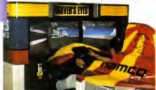
The adjustable seat is attached to a "Bodysenic" system. Players can physically experience the images and sounds on the screen through vibrations in the seat. The wheel and pedals are laid out the same as those in real F-1 cars.
